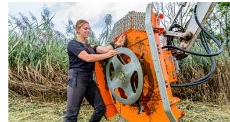
Easily replaced knives, replaceable attrition skids.
