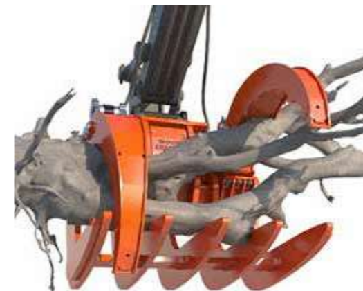
The gripper fingers adjust individually to the crop.
