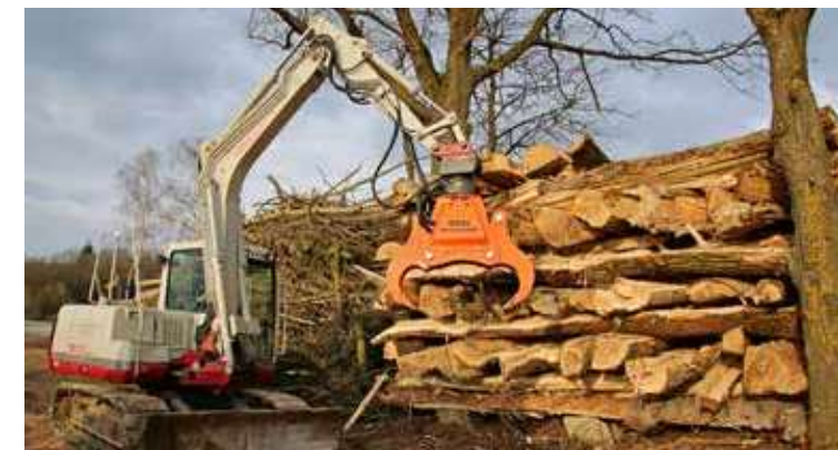
Pre-splitting wood allows a natural drying process.
